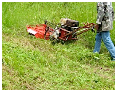
Walk-behind brush mowers are effective for small operations. 2
